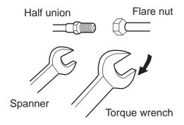
Forced fastening without careful centering may damage the threads and cause a leakage of gas.
